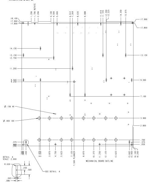
Figure 19. Mainboard Outline and Hole Location Drawing
